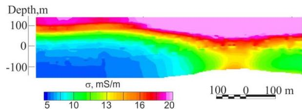
**Figure 8. Conductivity-depth image for frequency domain data: the target can be reliably pointed in the right side of section**
