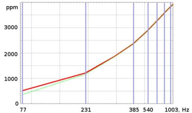
**Figure 7. Measured quadrature response (red) for 77 Hz is 150 ppm greater than modeled one over the same medium without deep conductor (green)**
