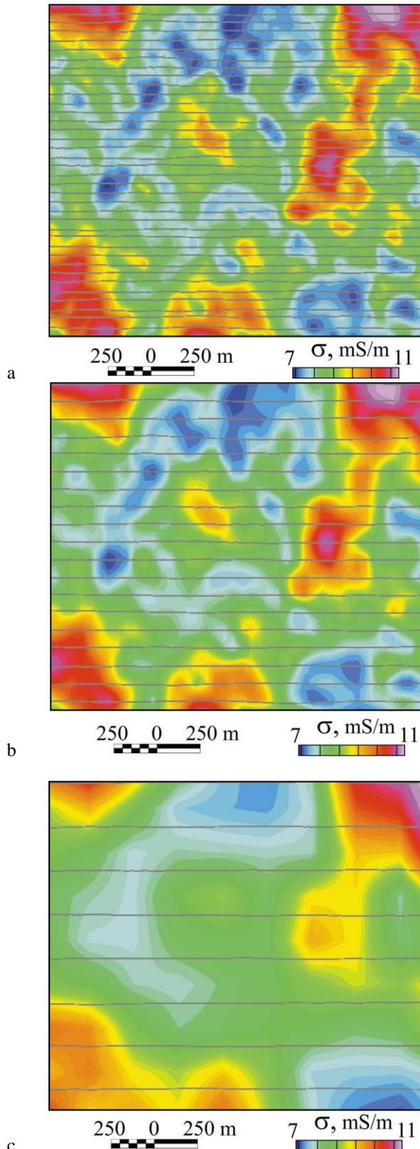
**Figure 3. Apparent conductivity after EQUATOR data processing a) 50 m between survey lines b) 100 m between lines (every 2<sup>nd</sup> line was used) c) 250 m between lines (only each 5<sup>th</sup> line was used)**
