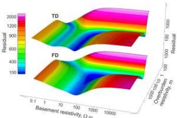
Figure 3. The residual (in ppb for FD and ppm/s for TD) of the calculated response for a two-layer medium model with varying basement and top layer resistivity for the model of 20 m layer of 100 Ω-m overlaying 80 Ω-m base.
