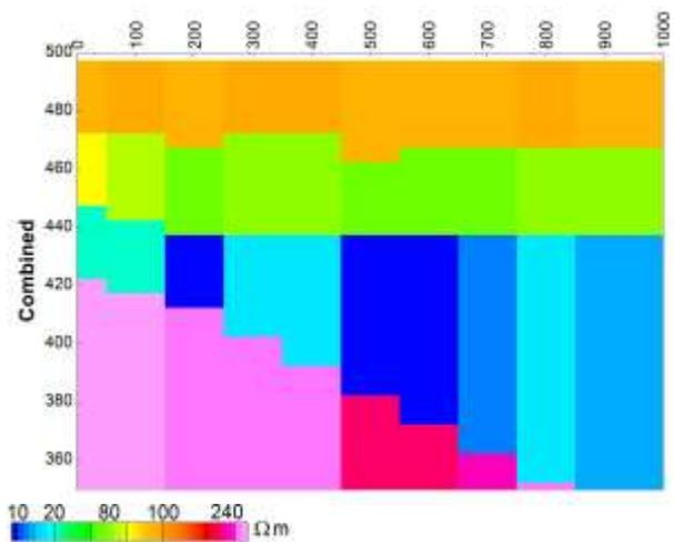
Figure 7. Combined 1D inversion of data acquired from 4-layer model data.
