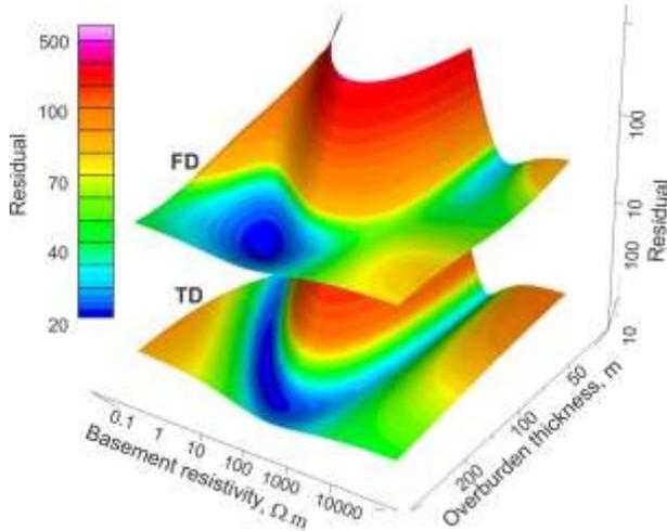
Figure 2. The residual (in ppb for FD and ppm/s for TD) of the calculated response for a two-layer medium model with a varying basement resistivity and top layer thickness and for the model (200 m of 2000 Ω-m overlaying 10 Ω-m).
