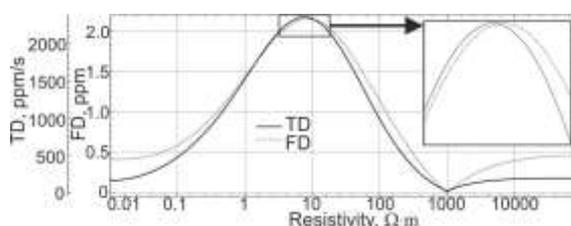
**Figure 1. The residual between the calculated response for a model of a homogeneous half-space with changing resistivity and response from the model of 1000  $\Omega\cdot\text{m}$  for TD and FD.**
