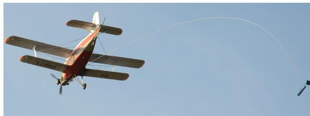
**Figure 1. General view of the airborne complex fitted with EM4H electromagnetic survey system**
