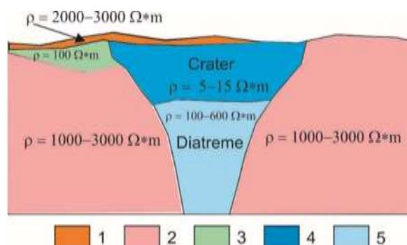
**Figure 1. Schematic geoelectric model of a kimberlite pipe for the Angolan shield. 1 – Kalahari Group; 2 – Archean Group; 3 – weathering crusts acc. to Archean Group; 4,5 – Crater and Diatreme Kimberlite Pipe**
