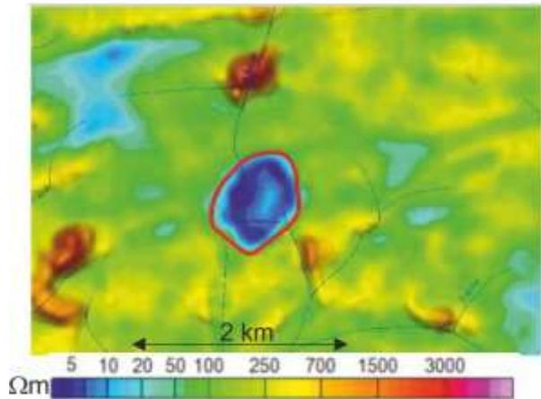
**Figure 3.** Resistivity map for 3163 Hz frequency channel for large (~ 1000 m) non-magnetic diamond kimberlite body (red circle) in Lunda Norte province (Angola).
