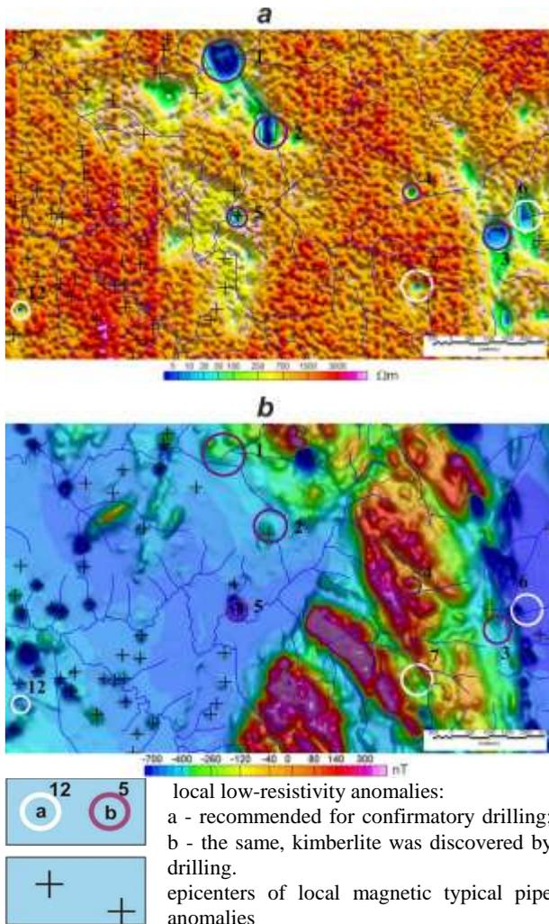
**Figure 5. Examples of kimberlite discovery according to the electrical prospecting and magnetometry data. a – apparent resistivity map for depth interval of 50-80 m; b – anomaly magnetic field map reduced to the pole.**
