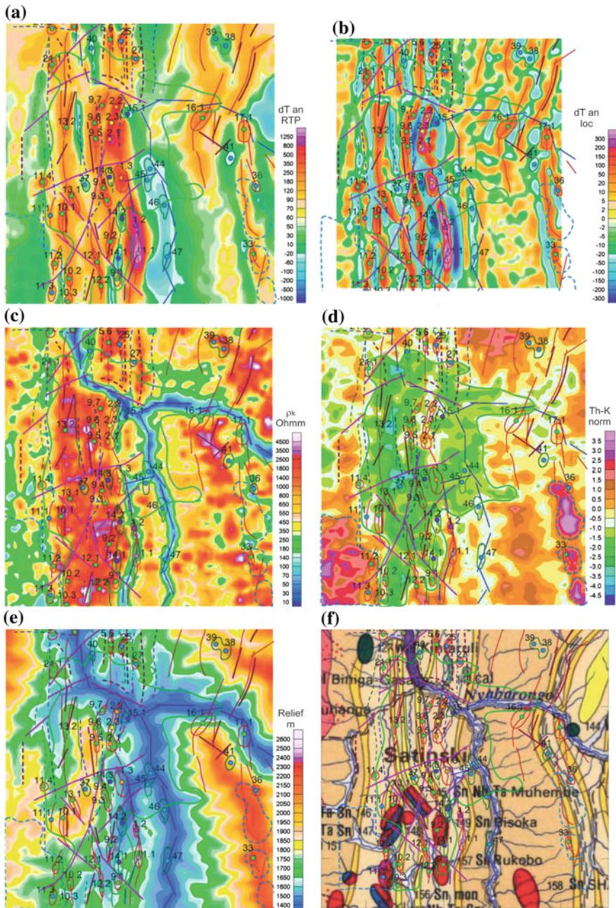
**Fig. 46.4** Results of airborne geophysical survey at a scale of 1: 25,000. **a** an anomaly magnetic field map reduced to the pole; **b** local part of anomaly magnetic field map; **c** apparent resistivity map for depth interval 0–30 m; **d** a map of the difference of the normalized concentrations of Th-K; **e** a map of the digital elevation model; **f** a fragment of the geological map
