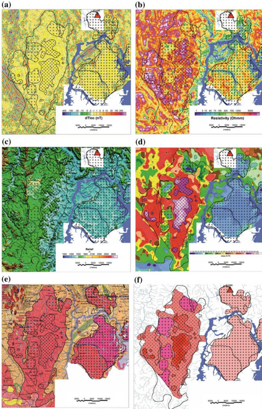
**Fig. 46.2** Mapping of granite intrusions according to the technology of EQUATOR: **a** local component of the magnetic field; **b** apparent resistivity at a time gate 5 mcs; **c** digital elevation model; **d** map of radiogeochimical specialization classes for K-Th; **e** geological map; **f** varieties of granites from the interpretation of airborne geophysical data
