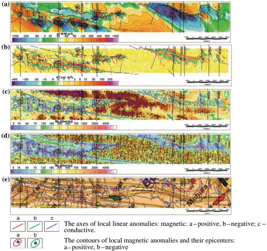
**Fig. 46.3** Example of infill survey at a scale of 1: 10,000: **a** magnetic field reduced to the pole; **b** local component of the anomaly magnetic field; **c** apparent resistivity map at a gate of 5  $\mu$ s; **d** map of apparent resistances for a window of 1000  $\mu$ s; **e** fragment of the geological map
