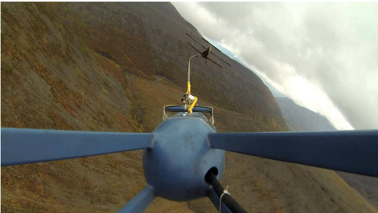
Fig. 8. The frequency-domain system with a non-rigid transmitter-receiver geometry EM-4H during the survey, 2014.
