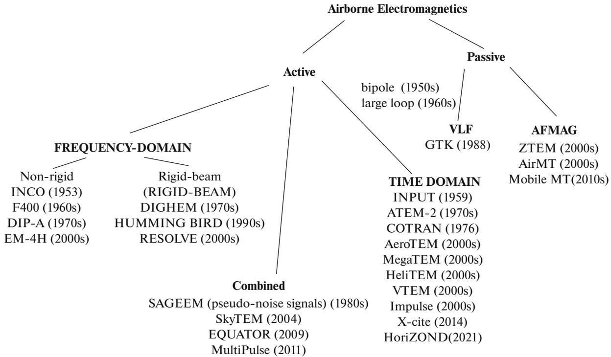
**Fig. 1.** A classification of basic airborne electromagnetic systems.
