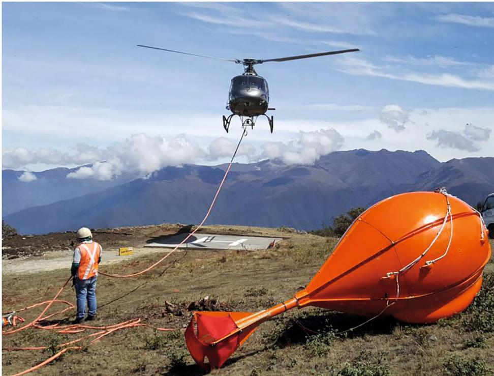
**Fig. 3.** The passive MobileMT system (Prikhodko et al., 2020).
