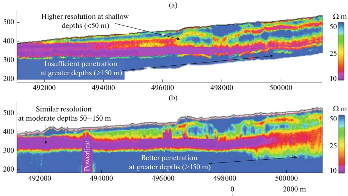
**Fig. 6.** Conductivity depth images constructed for (a) a frequency-domain system and (b) a time-domain system, illustrating differences and similarities in depth-resolution between systems (Chen et al., 2014).
