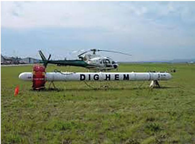
Fig. 7. The rigid-boom frequency-domain system DIGHEM.
