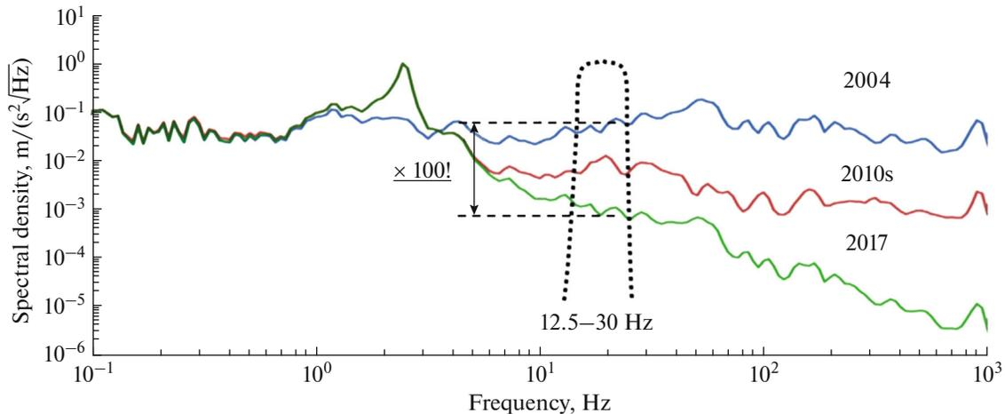
**Fig. 2.** Spectral density of measurements of noises in today's and previous generations of receivers (Sorensen, 2018).
