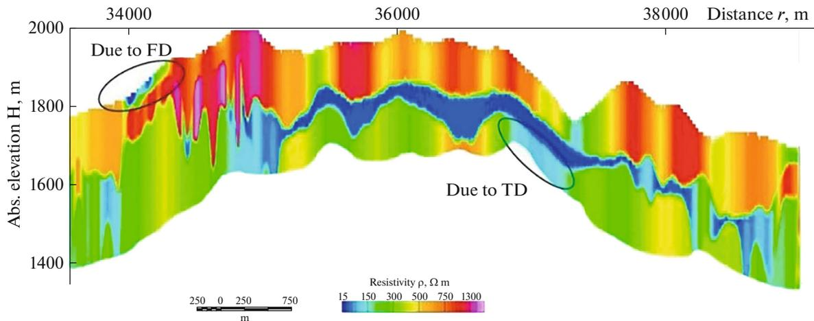
Fig. 14. Results of a combined (time-domain as well as frequency-domain) data inversion.
