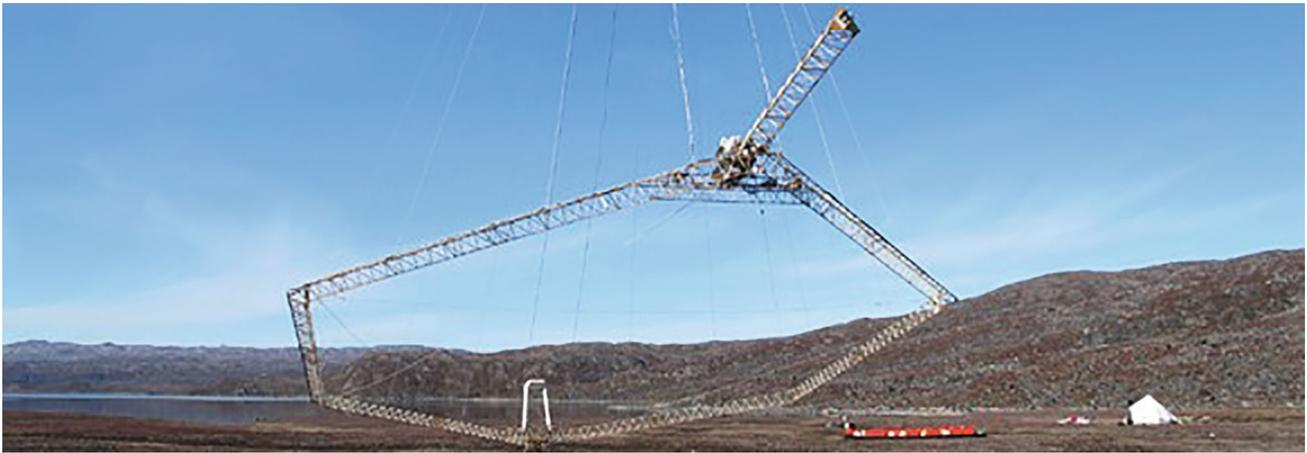
Fig. 9. The combined system SkyTEM.
