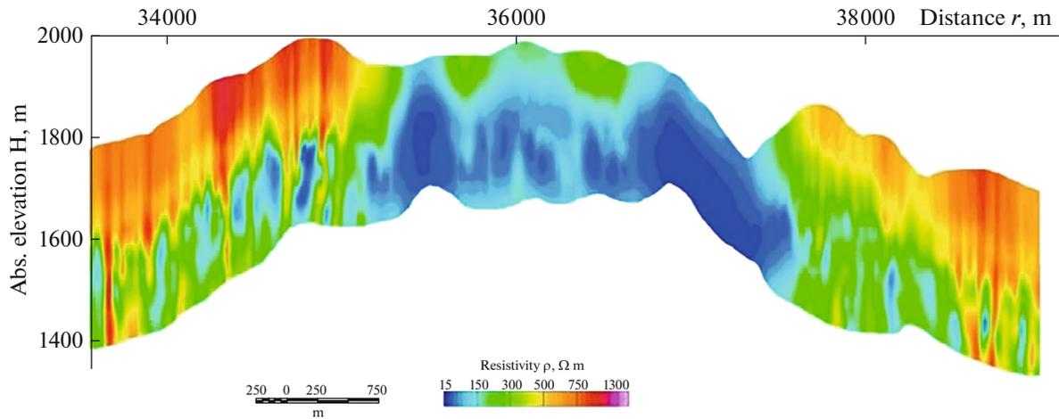
Fig. 13. A resistivity depth section constructed by time-domain data only.
