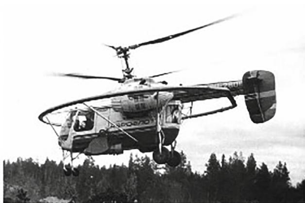
**Fig. 5.** An active system implementing the airborne transient electromagnetic method ATEM-2, 1970s.
