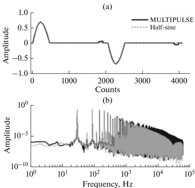
Fig. 10. (a) Signal waveform for MULTIPULSE and half-sine; (b) their spectra. The half-sine length is 4 ms, the peak—700000 Am<sup>2</sup>.
