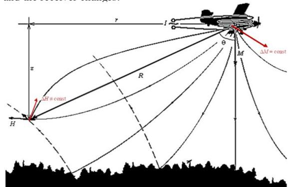
**Figure 1.** Airborne electromagnetic system EM4H. **R** - transmitter-receiver radius vector; **M** - vector of the magnetic moment of the exciting dipole;  $\Delta M$  - vector of the magnetic moment of the eddy current field; **H** - magnetic field vector of the exciting dipole;  $\Delta H$  - eddy current field vector.
