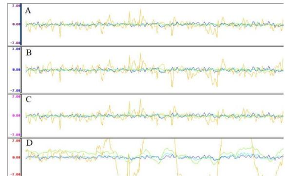
**Figure 6. Quadrature component for the EQUATOR at 4 frequencies. A - after compensation, with using the measurements of the parameters of two additional dipoles; B - using the 1<sup>st</sup> dipole, C - using the 2<sup>nd</sup> dipole, D - nulling.**
