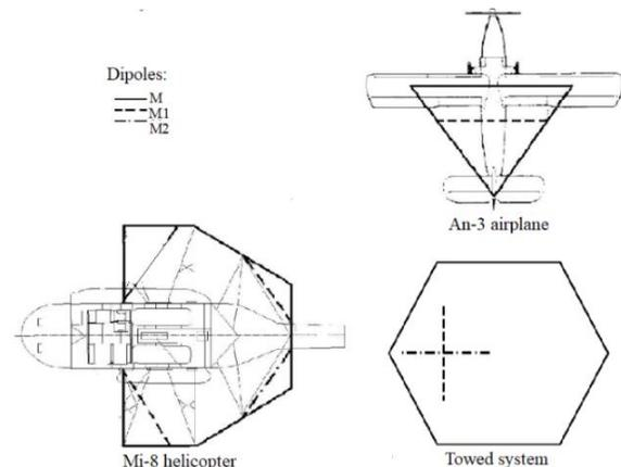
**Figure 2. Loops installation for EM4H modifications.**
