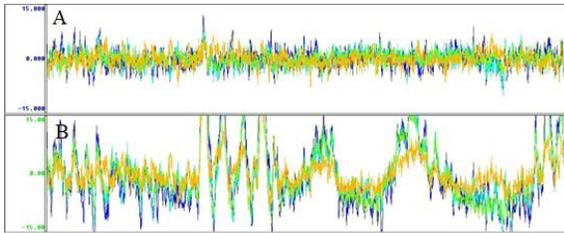
**Figure 4. Quadrature component for the An-3 aircraft at 4 frequencies. A - after compensation, with using the measurements of the parameters of the additional dipole; B - nulling.**
