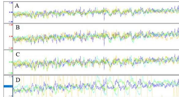
**Figure 5. Quadrature component for the Mi-8 helicopter at 4 frequencies. A - after compensation, with using the measurements of the parameters of two additional dipoles; B - using the 1<sup>st</sup> dipole, C - using the 2<sup>nd</sup> dipole, D - nulling.**
