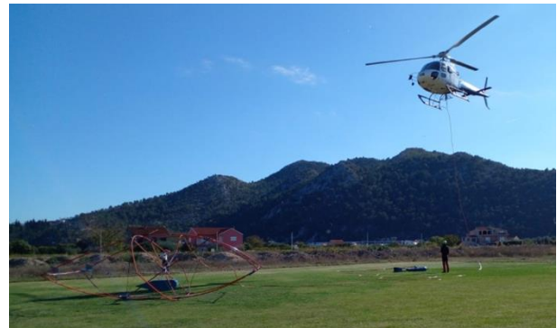
Figure 3. The AEM system EQUATOR during the Neretva survey in Croatia.
